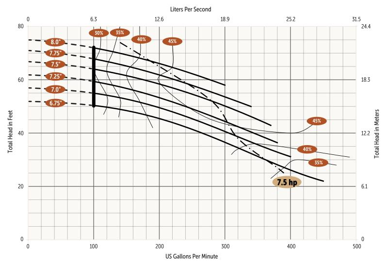
Stated efficiency values are hydraulic efficiency. Wire-to-Water (total) efficiency information is available upon request.
